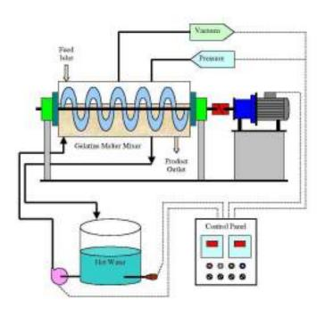
We offer automated gelatine melting systems for use in the manufacture of various gelatine products such as soft gelatine capsules. These systems are used for melting & keeping in fluid condition, the gelatine granules used in the process.
