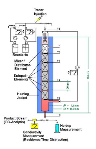
A trickle-bed reactor is employed to check for macrokinetic phenomena inside of catalystcontaining structured packings.
